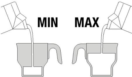
For optimum results, there are different measurement markings within the milk jug. The chart on the right shows the approximate number of cups produced at each of the measurement markings. This is a guide only as the frothing disc selected and the type of milk, for example whole milk (vitamin D), 2%, 1%, fat-free, half-and-half etc., can create different amounts of froth.
