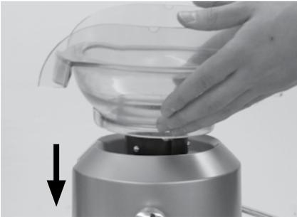
3. Align the arrows at the base of the stainless steel filter basket with the arrows on the motor drive coupling and push down until it clicks into place to create a secure fit with the motor base.
