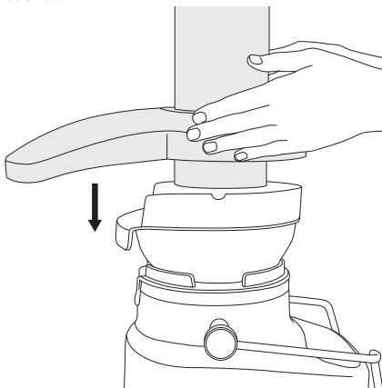
4. Raise the safety locking arm up and locate into the two grooves on either side of the juicer cover.
