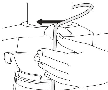
6. Slide the food pusher down the food chute by aligning the groove in the food pusher, with the small protrusion on the inside of the top of the feed tube.
