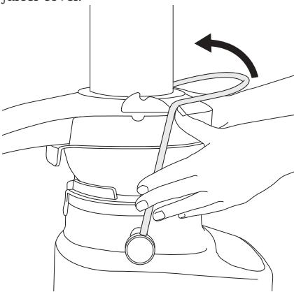
5. The safety locking arm should now be in a vertical position and locked into place on top of the juicer cover.
