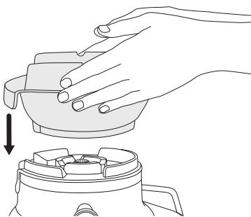
2. Align the arrows at the base of the stainless-steel filter basket with the arrows on the motor drive coupling and push down until it clicks into place to create a secure fit with the motor base.
