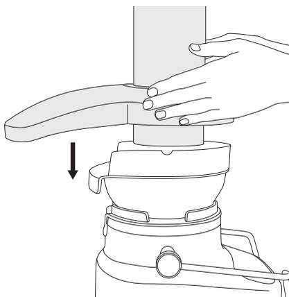
4. Raise the safety locking arm up and locate into the two grooves on either side of the juicer cover.
