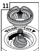
Push upper burr firmly into position
