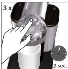
**5.** Push the button 3 times within 2 seconds. The button will blink quickly during the procedure. It will take less than 2 minutes before a flow comes out. The cleaning procedure will run automatically for 5 minutes. The procedure consists of 3 cycles of pumping water in/internal cleaning/water flowing from outlet to complete.
