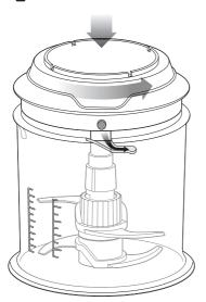
Align the tabs on the motor body with the grooves on the processing bowl cover to place the motor body on top. The motor body will be seated on the processing bowl cover ready for operation.
