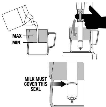
To start, touch the 'Milk' button. The screen will display the temperature of the milk as it heats. Milk texturing will stop automatically when the selected milk temperature is reached. Lift steam wand to remove milk jug. **Wipe the wand & tip with a clean damp cloth.** Lower steam wand to the down position and the wand will automatically purge.
