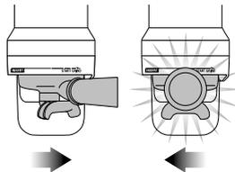
When the auto grind, dose & tamp function is complete, rotate the portafilter handle to the INSERT position and lower to remove.
