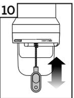
10 Clean grind outlet with grind outlet brush
