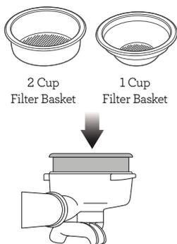
Use the 1 Cup Filter Basket for making a single cup or a weaker tasting espresso.
