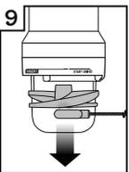
9 Remove tamping fan with tamp removal magnet
