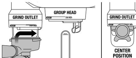
To start the auto grind, dose & tamp function, touch the Grind button on the display. Grinding will commence.
