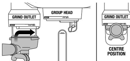
To start the auto grind, dose & tamp function, rotate the portafilter to the right then gently guide back to the centre position. Grinding will commence.
