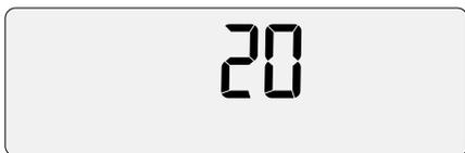
During this time, the machine will fill boilers with descale solution and heat to temperature. There may be some water flow through the group head during this time. Allow the countdown timer to reach 0 as this allows solution sufficient time to dissolve scale build up. However you can proceed to the next step at any time by pressing the 1 Cup button.
