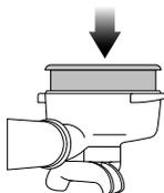
Use the 1 Cup Filter Basket for making a single cup or a weaker tasting espresso.
