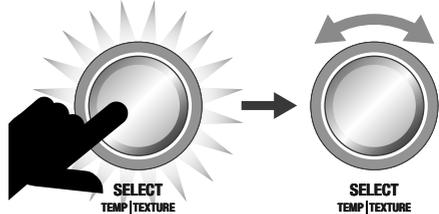
Press SELECT dial to set and the current polishing time will flash. Turn SELECT dial to select 2-10 seconds. Press SELECT dial to set. Machine will beep once to confirm settings.
