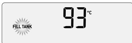
Fill tank with cold fresh water. The machine will not be able to make coffee or hot water while the tank is empty.
