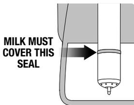
To start, press down and release steam lever. The LCD will display the temperature of the milk as it heats. Milk texturing will stop automatically when the selected milk temperature is reached. Lift steam wand to remove milk jug. **Wipe the wand and tip with a damp cloth.** Lower steam wand to the down position and the wand will automatically purge.
