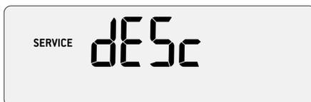
Please ensure you allow approximately 1.5 hour to complete the entire descale process and follow the step by step instructions. **If you've just finished using your machine, please ensure to turn the machine off and allow to cool for at least 1 hour before starting your descale process.**
