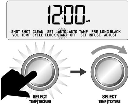
Turn the SELECT dial to the left or right to select the desired Auto Start time. Turning the SELECT dial faster or slower will change the rate of adjustment. When the required time has been reached, press the SELECT dial to set. A small clock icon will be displayed on the LCD when the Auto Start function has been programmed.
