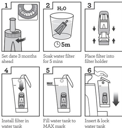
The provided water filter helps reduce the risk of scale build-up in and on many of the inner functioning components. Replacing the water filter every three months will reduce the need to descale the machine. If you live in a hard water area, it is recommended to change the water filter more frequently.
