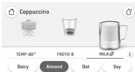
Milk texturing will stop automatically when the selected milk temperature is reached.
