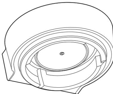
7. Re-insert the dispersion plate, then the shower screen, then the screw. With your fingers, turn the screw clockwise for 2-3 revolutions and use a flat screw driver to tighten until the screw is flush with the shower screen.
