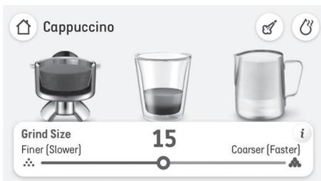
The grind size will affect the rate of water flow through the coffee in the filter basket and the flavour of the espresso. When setting the grind size, it should be fine but not too fine and powdery.
