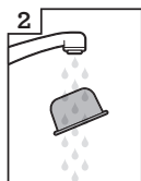
Rinse water filter
