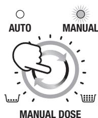
Press the MANUAL DOSE button to switch to manual dose mode. The light around the MANUAL DOSE dial and the MANUAL light will illuminate when in manual mode.
