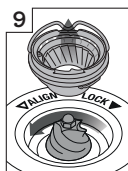
Push upper burr firmly into position
