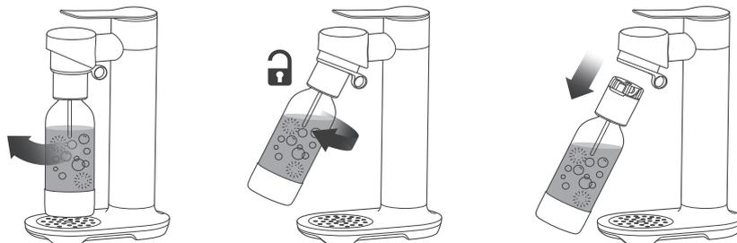
4.3 EN Use the ring to pull the tilt head forward.
